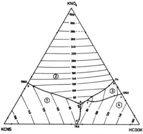
Fig. 2. Map of the liquids area of the K(CNS, HCOO, NO<sub>3</sub>) ternary system.
