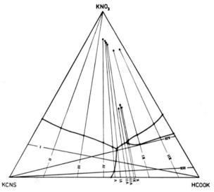
Fig. 1. Cuts in the K (CNS, HCOO, NO<sub>3</sub>) ternary system.
